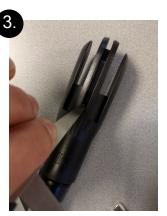
Use a pair of small flat head screw drivers to simultaneously depress both toggles and slide head off.
